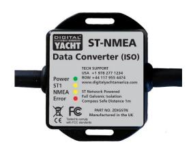
As data starts to be received from the SeaTalk network or on the ISO interface (from the computer) the Yellow "ST1" and "NMEA" LEDs will flash. If they are not flashing, then no data is being received on that interface.
