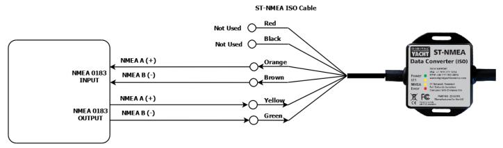
EQUIPMENT WITH TWO WIRE NMEA 0183 CONNECTIONS (e.g. Raymarine, Navico, etc.)
